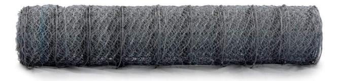
The hexagonal IS 16014 mesh type and rope spacing is designed to provide various strengths reaching upto 200 kN/m. StrongNet has an excellent 'fall' during installation due to the vertical wire ropes and provides excellent function as a 'drapery' mesh system. The double twist of the hexagonal mesh prevents unravelling of the netting if a wire gets cut due to any reason.
